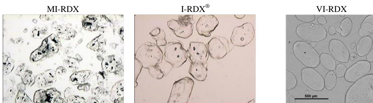
Figure 1: Optical microscopy with matching refractive index of MI-RDX, I-RDX ® and VI-RDX
