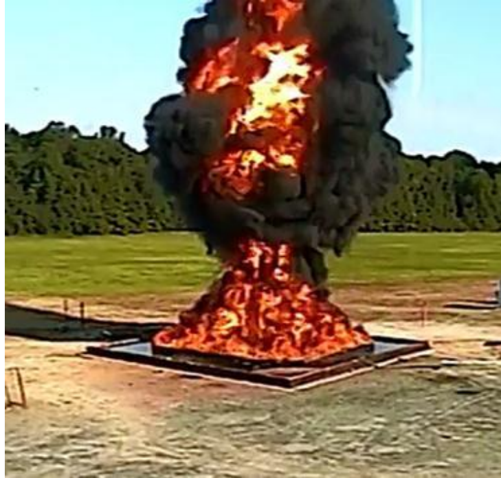
Figure 1. Fast Cookoff Test with Kerosene Based Fuel.
