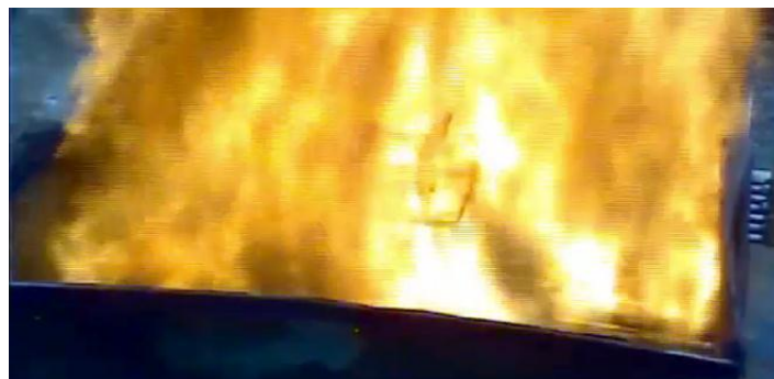
Figure 8. Photograph of Propane Flame with 81-mm Mortar with CompB Explosive Fill Looking Down on Flame.
