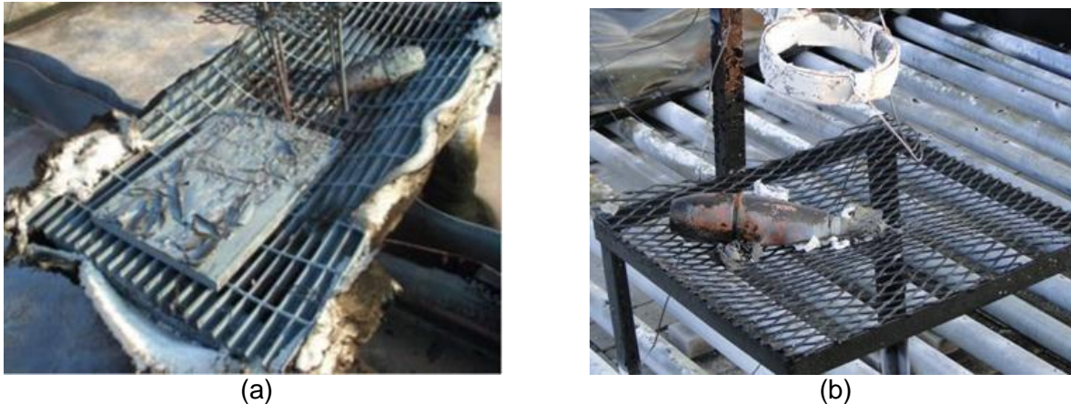
Figure 4. Post-test Photograph of 81 mm Mortar with IMX-104 Explosive Fill-Fast Cookoff Test. (a) Jet-A Pool Fire, (b) Propane Fire.
