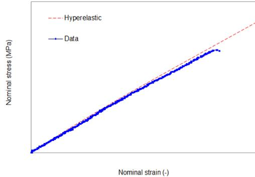
Figure 5: Example Hyperelastic Function Fitted to Model
