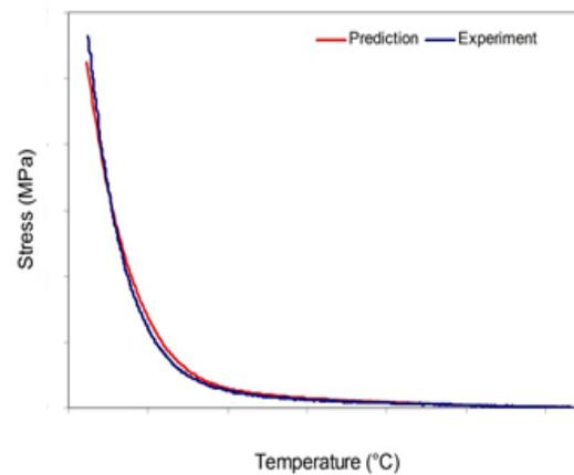
Figure 10: Stress vs Temperature during Simultaneous Straining and Cooling
