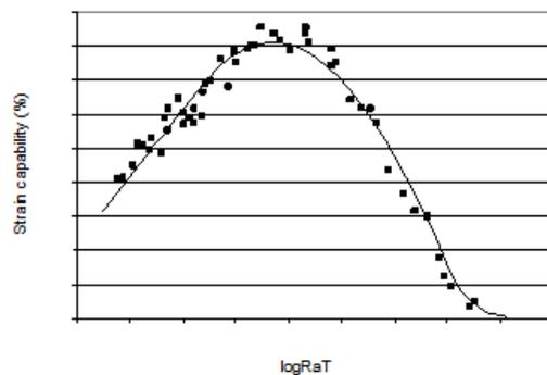
Figure 12: Example Failure Envelope for Strain Capability
