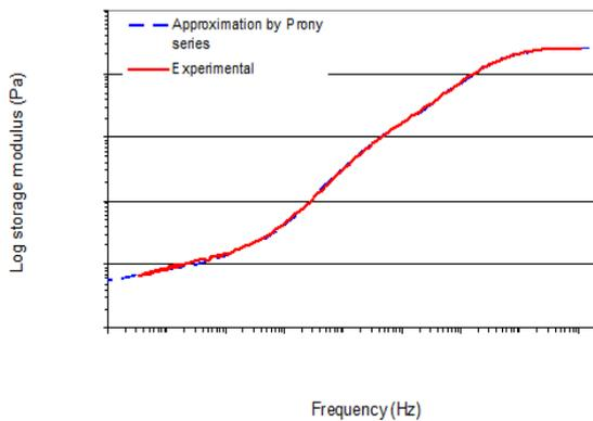
Figure 4: Example Storage Modulus fitted with Prony series
