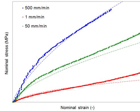
Figure 7: Experimental and Model Predictions for Cold Analysis
