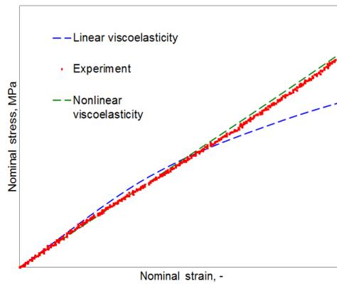
Figure 8: Comparisons between Linear and Nonlinear Viscoelastic Models
