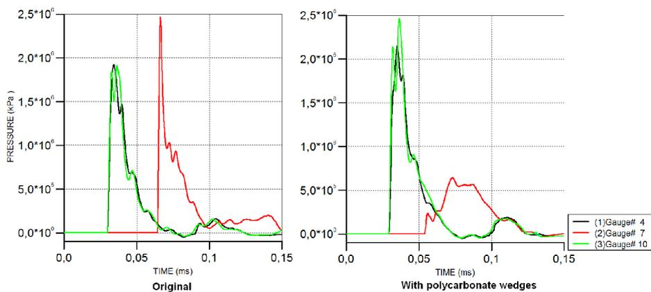
**Figure 10.** Pressure loads with the original design compared to with the protective wedges.
