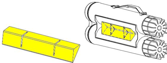
**Figure 8.** Pressure reducing wedges.
