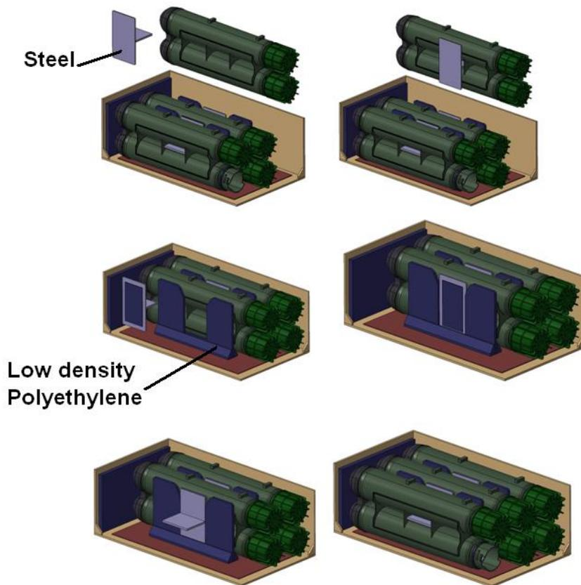
**Figure 19.** Packaging arrangement for the final testing.
