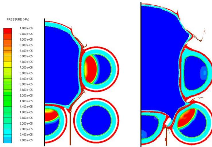
**Figure 6.** Pressure distribution at times 45 and 75  $\mu$ s after initiation.
