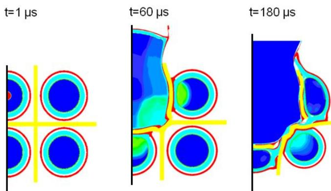
**Figure 12.** Pressure fringes in the rounds at three times after initiation.
