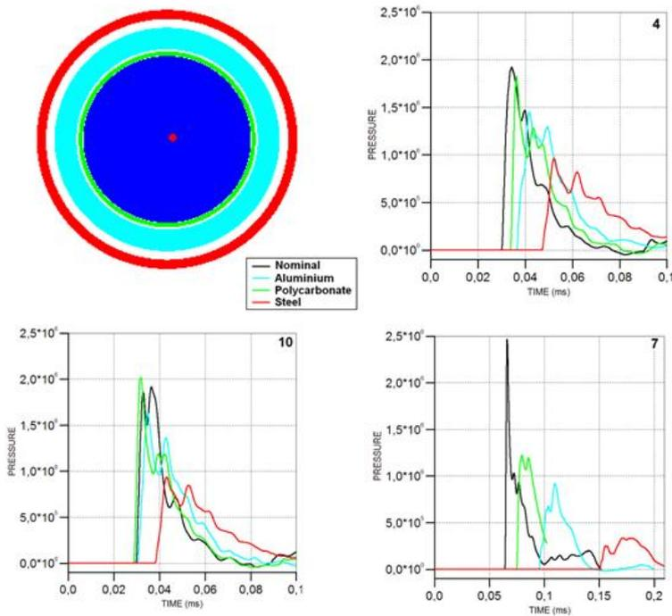
**Figure 13.** Pressure (kPa) as a function of time in the studied gauge points for three different cross materials compared with the set up without any protection.
