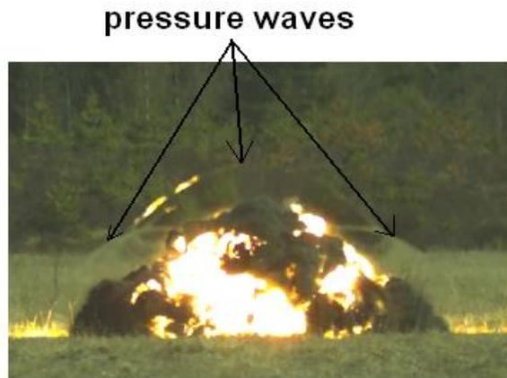
**Figure 2.** More than one pressure wave in the air indicating an unacceptable test result.
