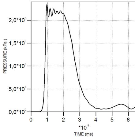
**Figure 4.** The simulated pressure as a function of time in the explosive at the limiting impact velocity for detonation.
