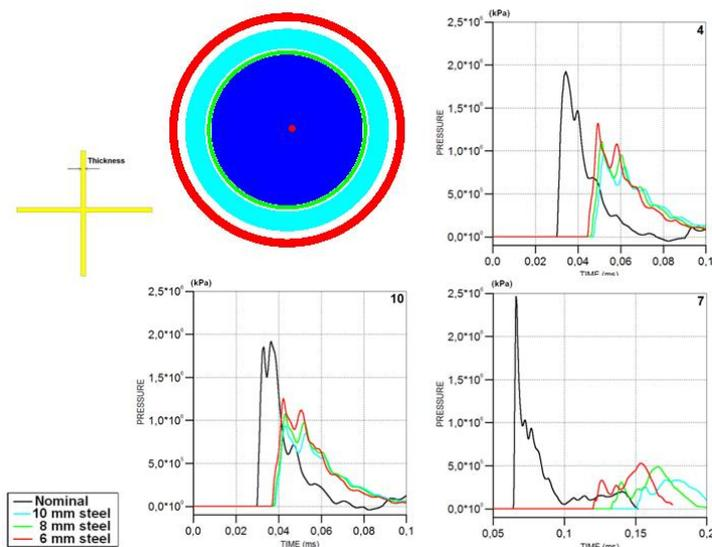
**Figure 14.** Pressure as a function of time in the studied gauge points with steel thicknesses 10, 8 and 6 mm steel.
