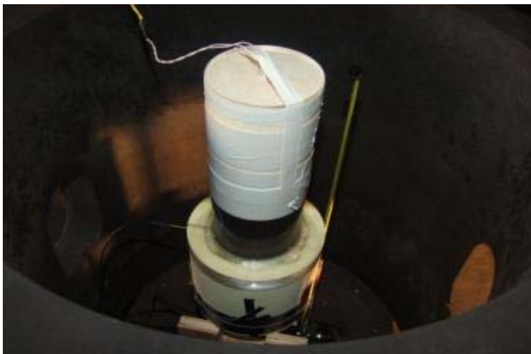
Figure 7. Example of 2D Corner Turning Test Setup
