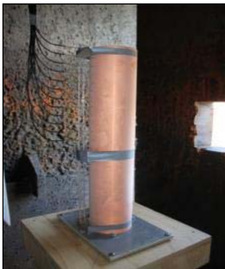
Figure 3. Four Inch Diameter Cylinder Expansion Test Setup
