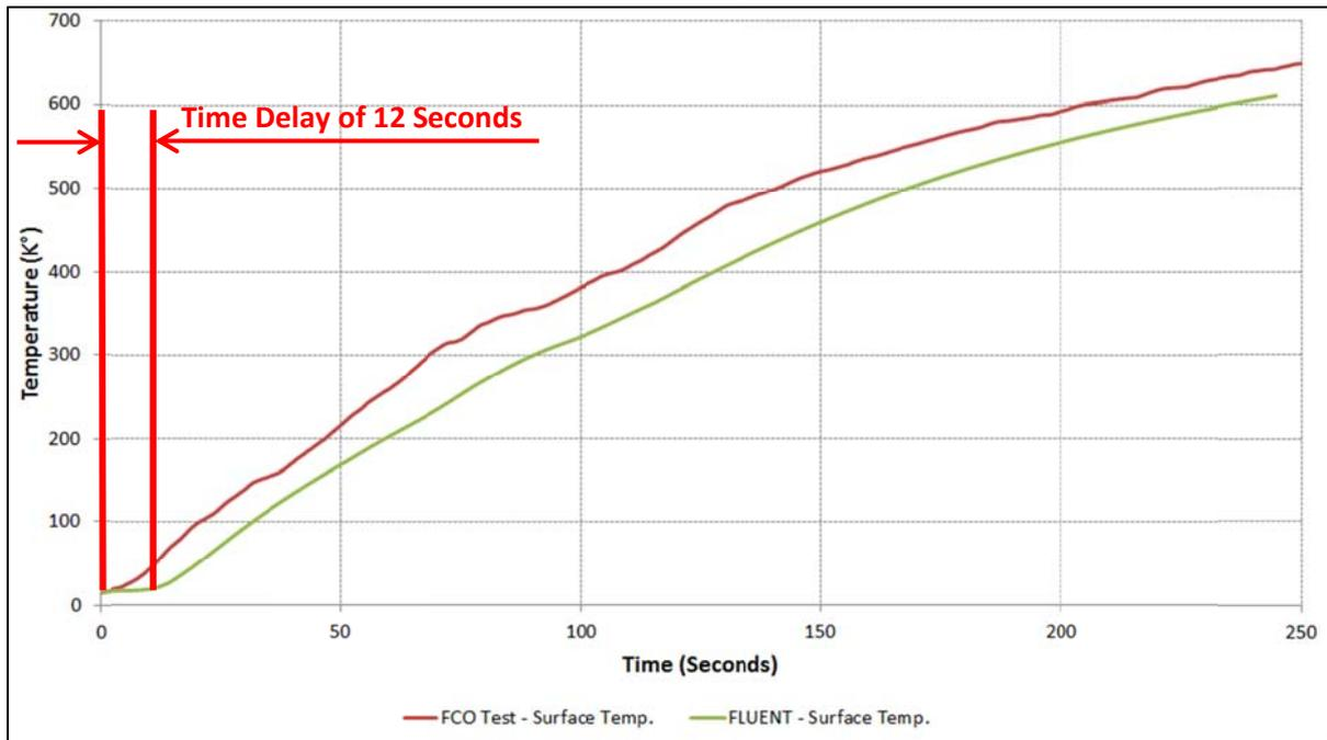
**Figure 5. Surface Temperature Comparison of Test and Numerical Results - Test Case**
