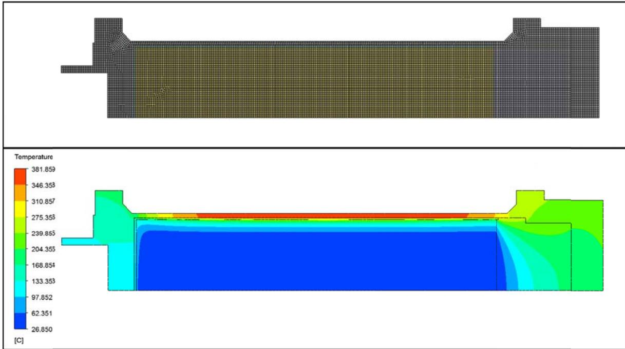
**Figure 6. Mesh Construction (top) and Temperature Gradient (bottom) of Test Items 7-8**
