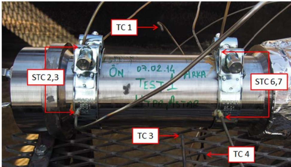
**Figure 2. Thermocouple Placement on 1<sup>st</sup> Test Item**
