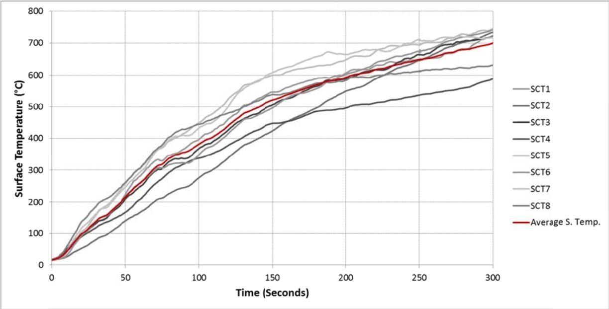
**Figure 4. Surface Temperature Readings from the 1st Test Item**
