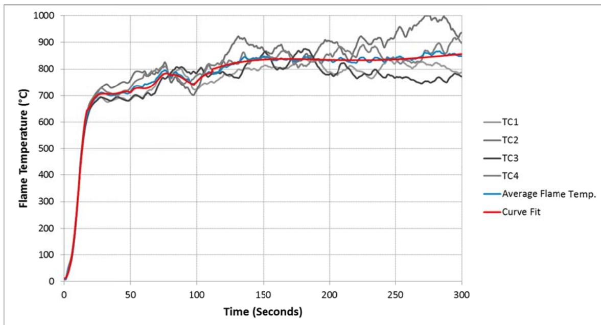
**Figure 3. Flame Temperature Readings from the 1<sup>st</sup> Test**
