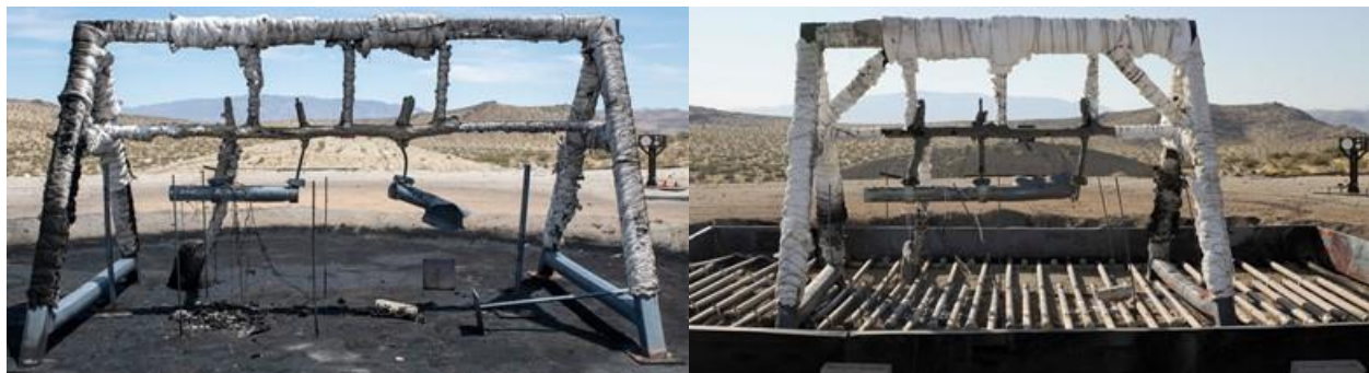
Figure 9. FCO posttest for identical rocket motors. Motor on left tested with liquid-fuel pool fire. Motor on right tested with propane burner.
