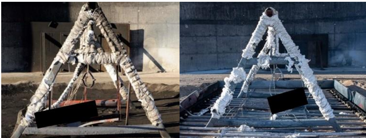
Figure 3. FCO posttest for identical test items. Item on left tested with liquid-fuel pool fire. Item on right tested with propane burner.
