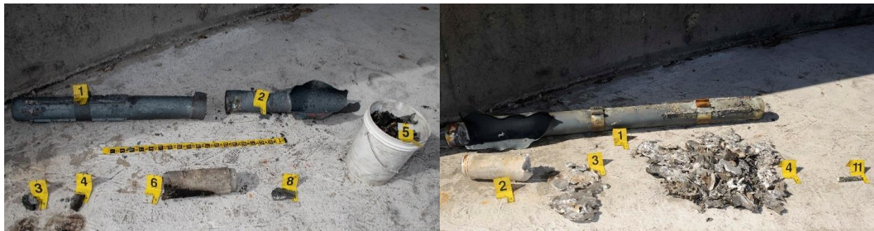
Figure 10. FCO posttest rocket motors remains. Motor on left tested with liquid-fuel pool fire. Motor on right tested with propane burner.
