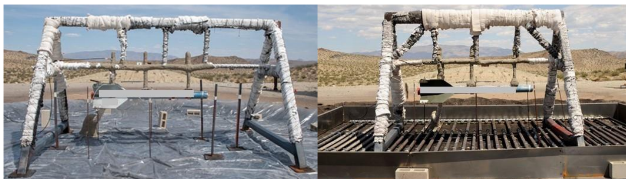
Figure 4. FCO setups for identical rocket motors. Motor on left tested with liquid-fuel pool fire. Motor on right tested with propane burner.
