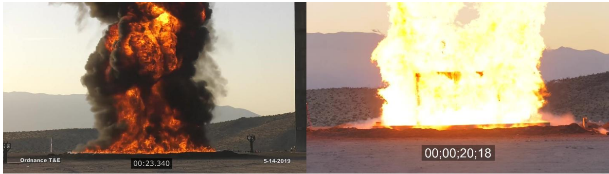
Figure 8. Fully developed flames before reaction, left photo of liquid-fuel pool fire and right photo of propane fire.
