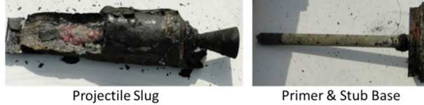
Figure 13. Test Item Remains Removed from the Shipping Container, Slow Cook-Off Test
