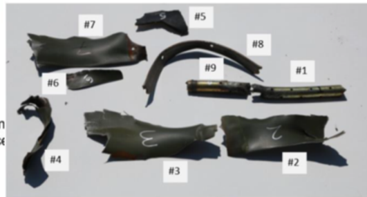
Figure 5. Test Item Remains Recovered at a Range Greater than 50 Feet from the Test Stand
