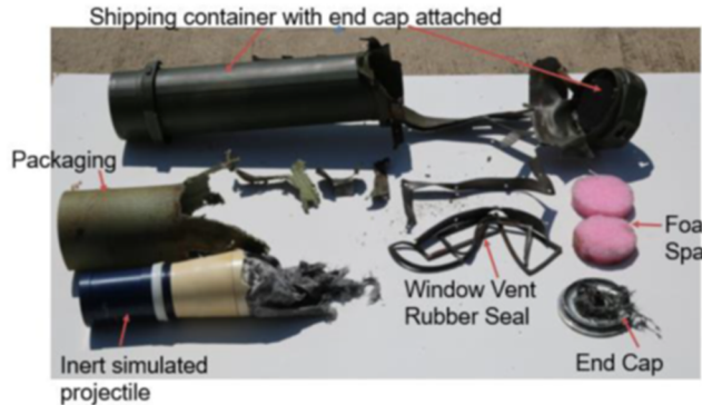
Figure 4. Test Item Remains Recovered within 50 Feet of the Test Stand, Fragment Impact Test
