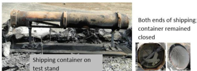
Figure 12. Post-Test Condition of Test Item Container, Slow Cook-Off Test
