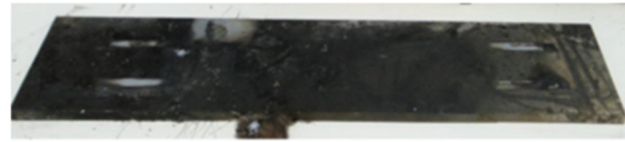
Figure 14. Post-Test Condition of Witness Plate, Slow Cook-Off Test
