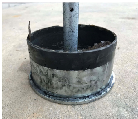
Figure 17. Post-Fire Stub Base
