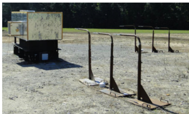
Figure 10. Photograph of completed test Setup, Slow Cook-Off Test
