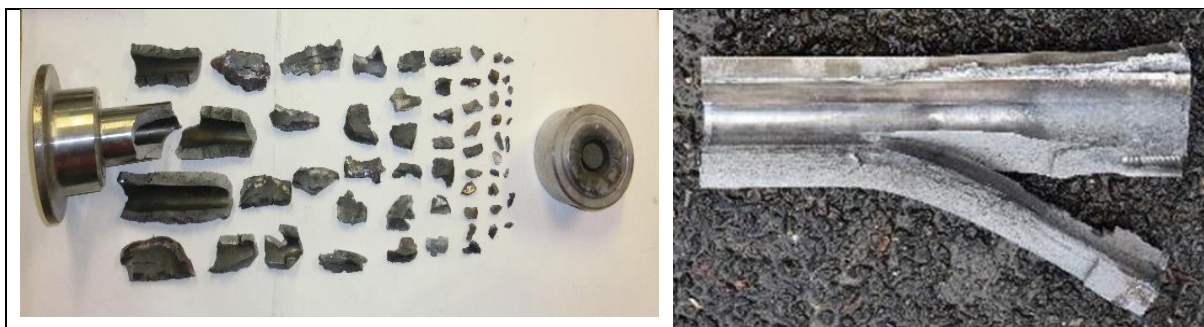
Figure 3. Still images of the recovered remnants from two experiments. Left image is from an experiment using 20 mm wall thickness steel tube and the right image is from a steel vessel with a quartz window.
