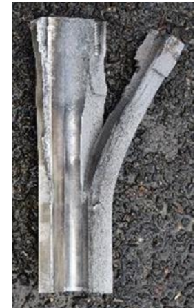
Post test Quartz window Vessel remnant
