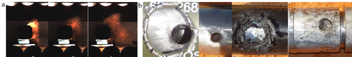
Figure 12. 0.1875" Hardened Steel Container PIMS (RT18597) (a) HSV at 311 \mu s, 2101 \mu s, 4202 \mu s from impact; (b) Recovered debris and intact warhead
