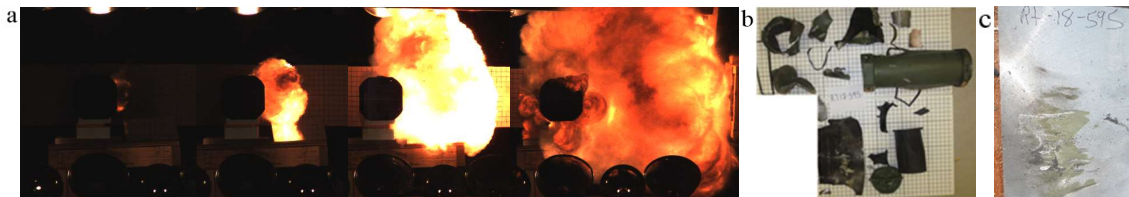
Figure 11. 0.25" 6061 Aluminum Container PIMS (RT18595) (a) HSV at 310 \mu s, 895 \mu s, 1517 \mu s, 2101 \mu s from impact; (b) Recovered debris; (c) Witness plate gouging
