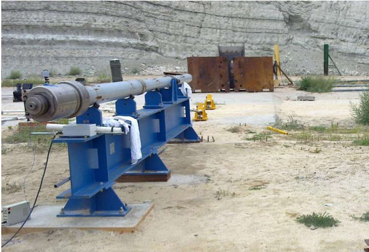
Figure 12. 50 mm powder cannon used in the fragment impact test.
