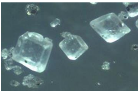
Figure 2 wax 1.2% graphite 0.6% Pressed density 1.77 g/cm 3 at 30 bar HMX
