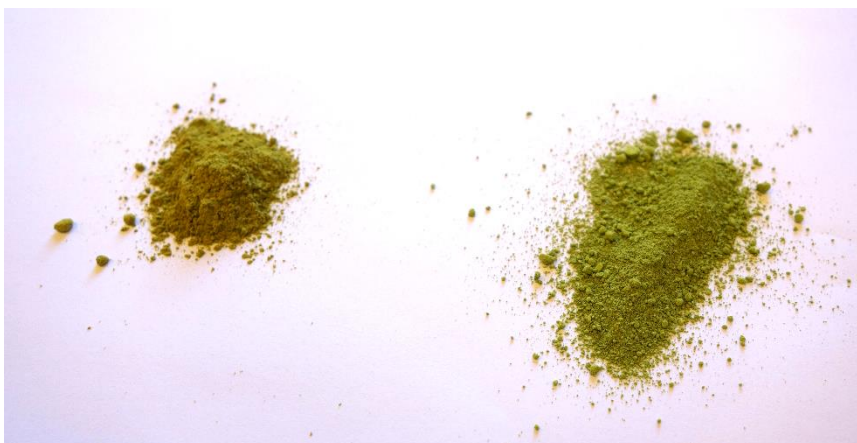
Figure 5 Photo of the two synthesized samples, lower (to the left) and higher (to the right) temperature.
