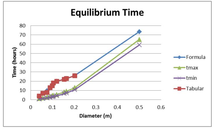
Calculated time for a Composition B cylinder center to reach 45°C compared to the tabular and formula based guidance in STANAG 4224.
