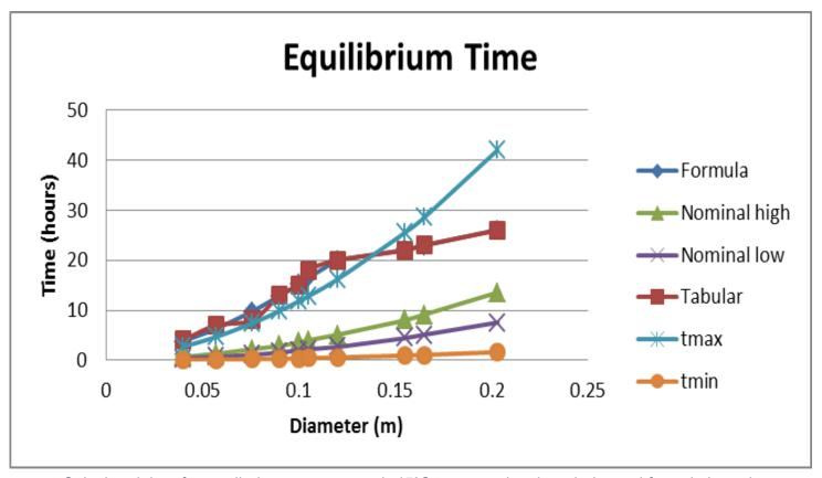
Calculated time for a cylinder center to reach 45°C compared to the tabular and formula based guidance in STANAG 4224.
