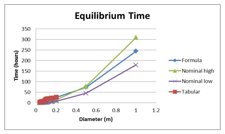
Calculated time for a cylinder center to reach 45°C compared to the tabular and formula based guidance in STANAG 4224.
