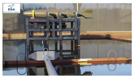
The reaction started approximately 4 minutes after the beginning of the test. The explosive material burned during 11 minutes.
