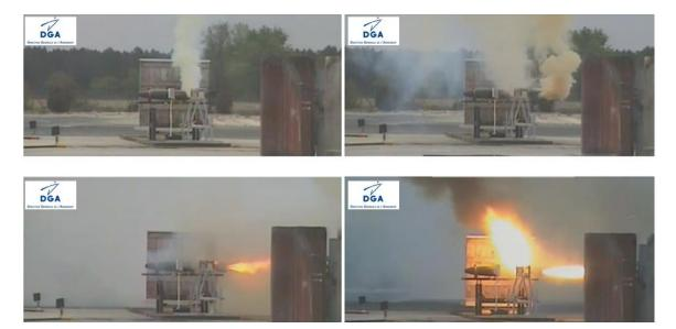
At the end of the test, the bomb body was found at its location, with no damage to the structure. No projection of fragment nor significant overpressure were recorded.
