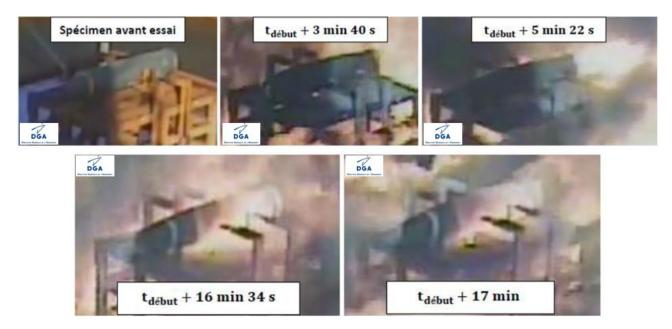
At the end of the test, the bomb body was found at its original location, with no damage to the structure. No projection of fragment nor significant overpressure were recorded.
