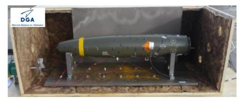
A reaction was observed at 35 h after the start of the 3.3 °C/h slope, at an average measured temperature of 161.5 °C.
