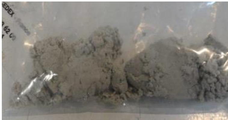
Figure 5: Sample after 14 days hydrolysis treatment, washing and drying steps
