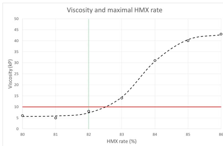
**Figure 3:** Viscosity and maximal HMX rate evolution
