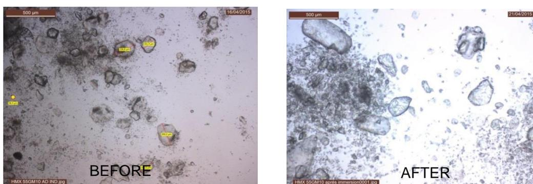
Figure 2: Pictures of HMX before and after hydrolysis
