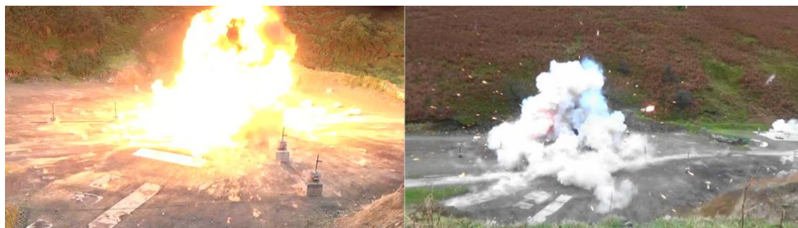
Typical response of refractory filled rocket motor [left] and Roxel's IM Rocket Motor [right] to Sympathetic Reaction trial
