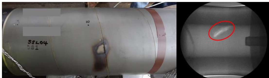
Typical example of case scorch mark following static firing [left] and charge damage observed on Real Time X-ray (RTX) during a static firing [right]
