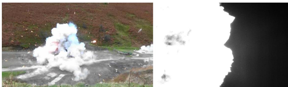
'Low' SiC% Response [left] and acceptor motor engulfed by donor blast [right]
