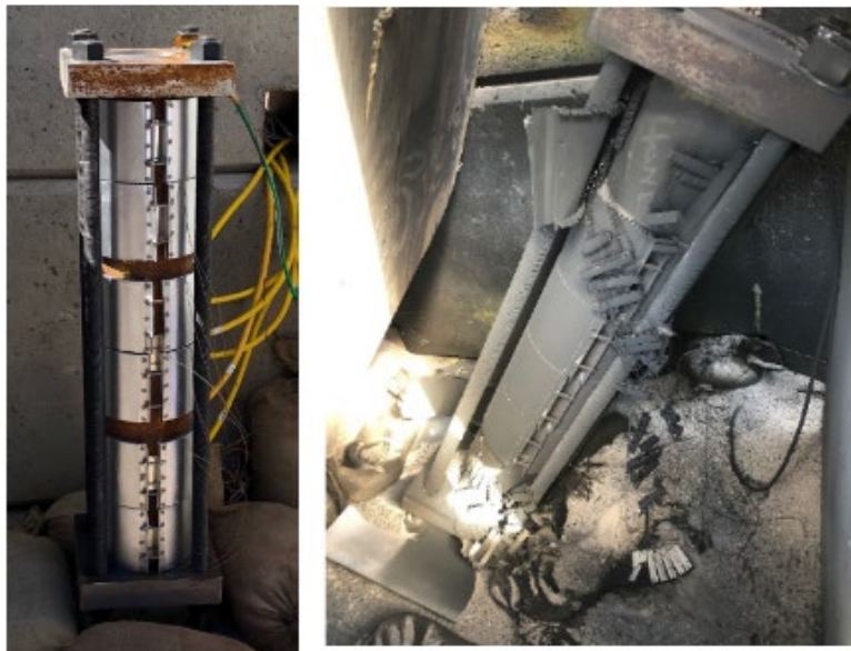
Figure 5. Steel test article before and after firing
