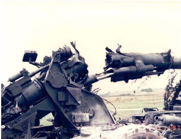
Figure 1: The in-bore detonation of a 155mm artillery round killed two Singaporean soldiers during a training exercise in New Zealand in 1997. The cause of the accident was determined to be a defective fuze. [1]
