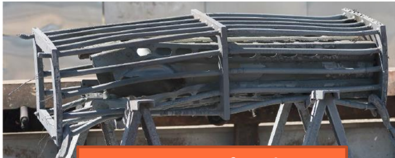
V127BER cage after the test
