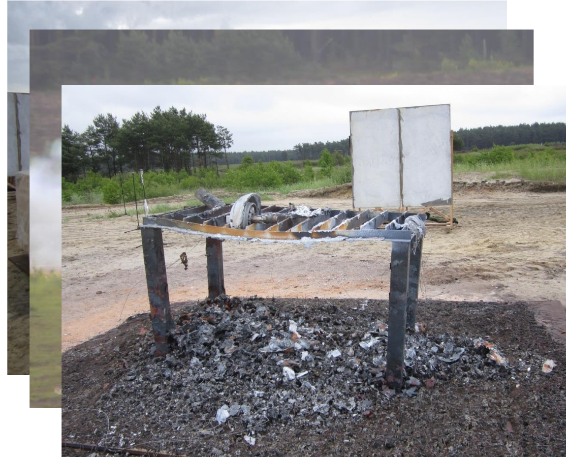
CM108 Sympathetic Charge Assessment: Type V (Burning)
