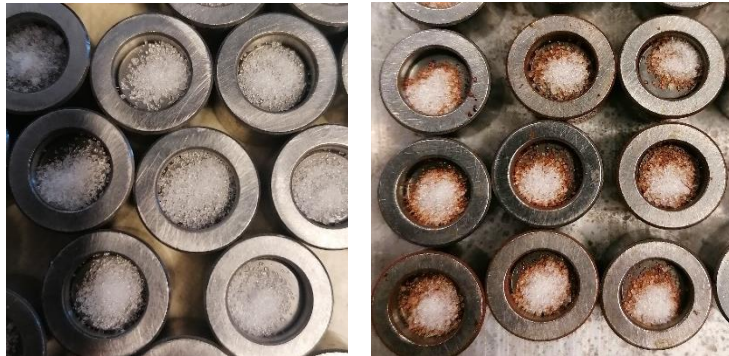
Figure 10: AP samples before (left) and after (right) conditioning at 90% RH in the test apparatus.
