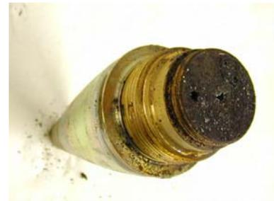
Diagram 12 : PDM557 fuze after SCO test
