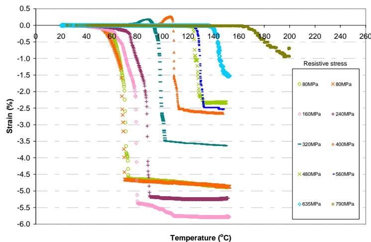
*Figure 5: Set of test results for Ti Ni wire contracting against various resistive stresses*
