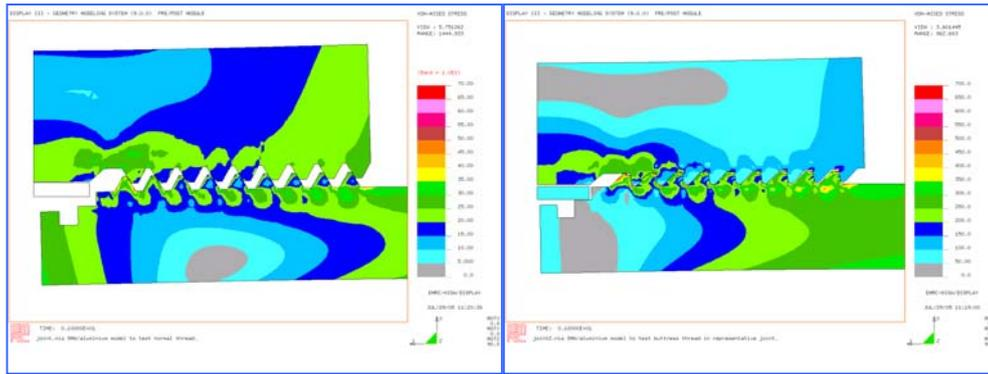
Figure 1: Elastic-plastic FE model of a) a standard ISO thread and b) an equivalent buttress thread. It is evident that the IOS thread has a strong tendency to spring apart under load, whereas the buttress thread largely avoids this.
