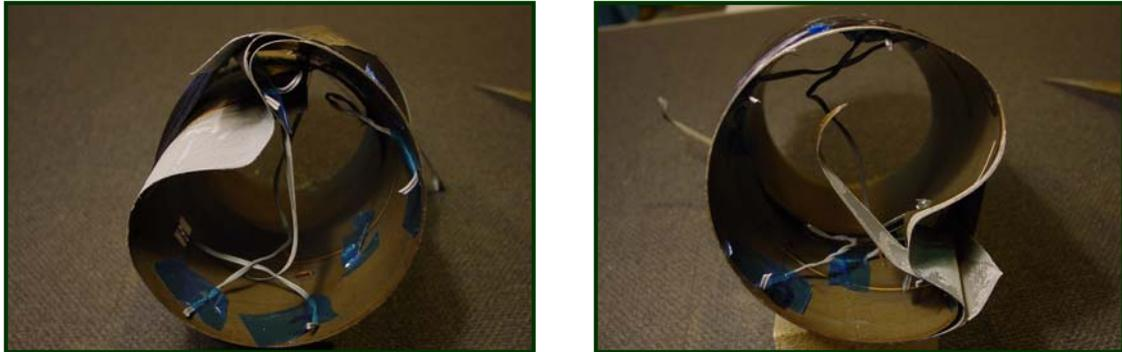
*Figure 10: A buckled and cracked section of a steel strip laminate rocket motor case*
