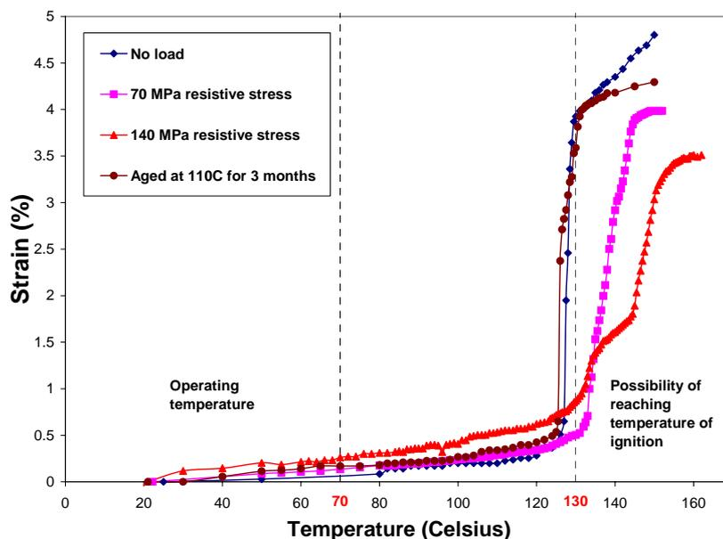
Figure 2: Results of strain recovery tests on short Ti Ni rods upon heating
