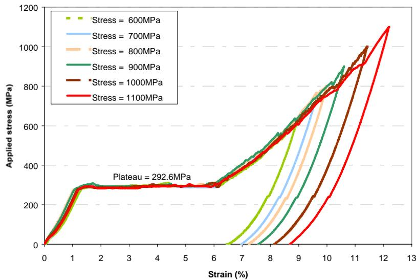
Figure 4: Stress-strain curves measured for Ti Ni SMA wire in a standard tensile testing machine
