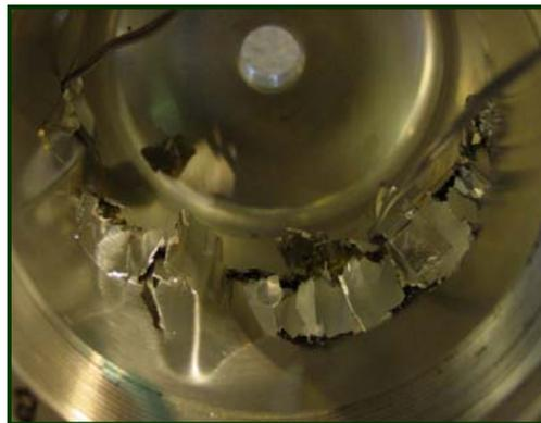
*Figure 6: Successful demonstration of a cutting device on a NLAW flight motor case*
