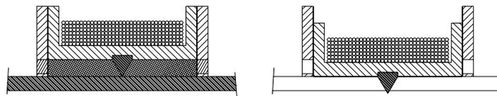
*Figure 3: Schematic diagram showing cutters being driven into a rocket motor case by the contraction of SMA wire*
