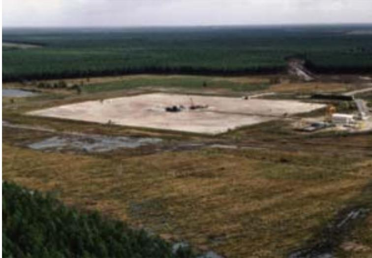
CAEPE operates 3 safety zones that are free from any obstacles over 200m x 200m. Each one is equipped with underground instrumentation and able to accommodate up to 135 measurements.
