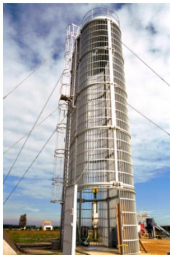
A new drop test tower has been recently built which allows dropping from up to 12 m for a test article weighing up to 2.2 tonnes. The cage surrounding the drop test improves the safety conditions of test.
