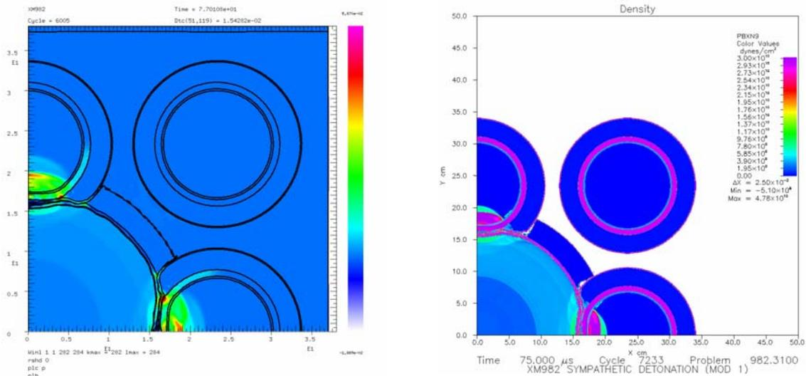
**Figure #6 (U) CALE and HULL pressure distributions**
