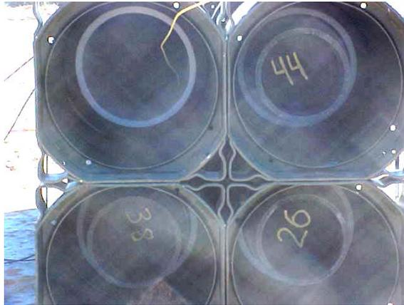
**Figure #1 (U) Initial test packaged rounds without end caps**
