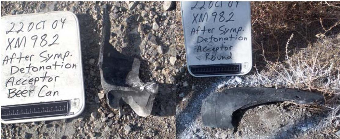
**Figure #11 (U) Large warhead case fragments after SD testing (base and vents)**
