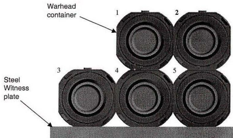
**Arrangement of Test Assemblies (End View)**
