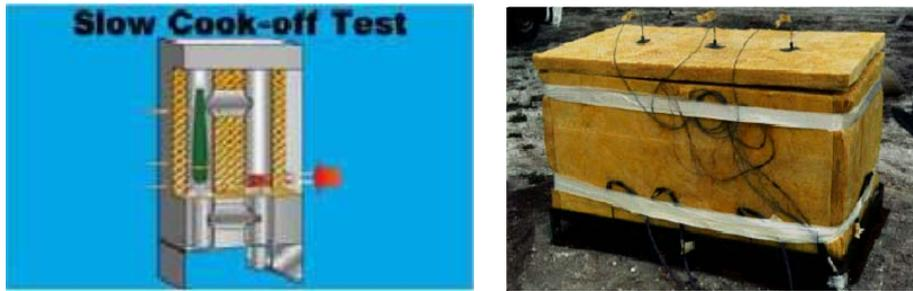
**Figure 4 – Examples of SCO Test Configurations**
