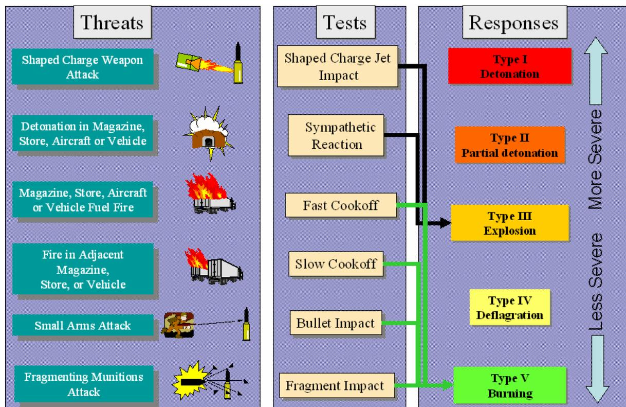
Figure 10 – Tests and reaction Levels [10]
