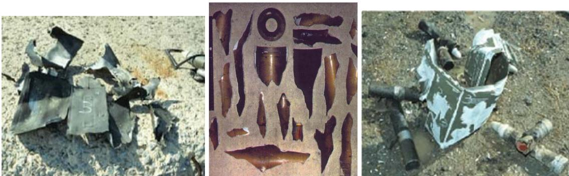
**Figure 8 – Results Examples of a Type III Reaction**
