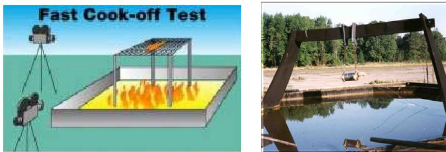
**Figure 5 – Examples of FCO Test Configurations**
