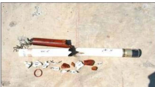
**FIGURE 8. Composite Case Debris**
