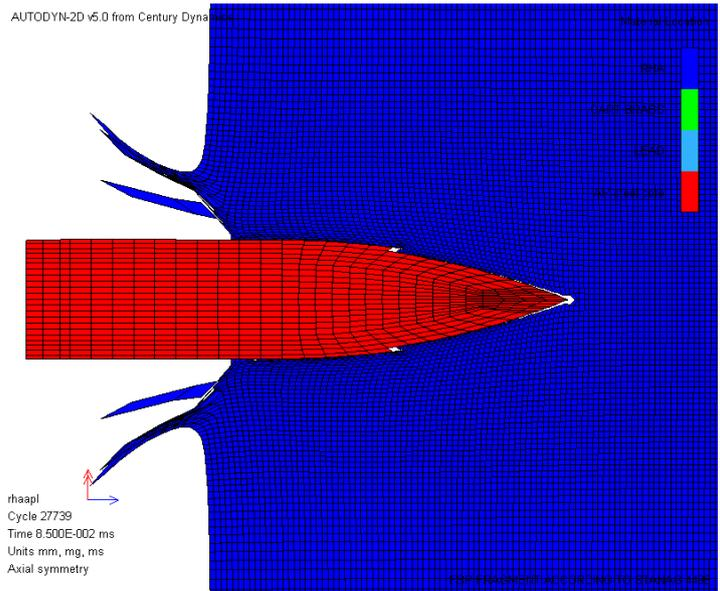
Figure 4: AUTODYN-2D screen-shot of 0.5" M2 AP round impacting thick RHA.
