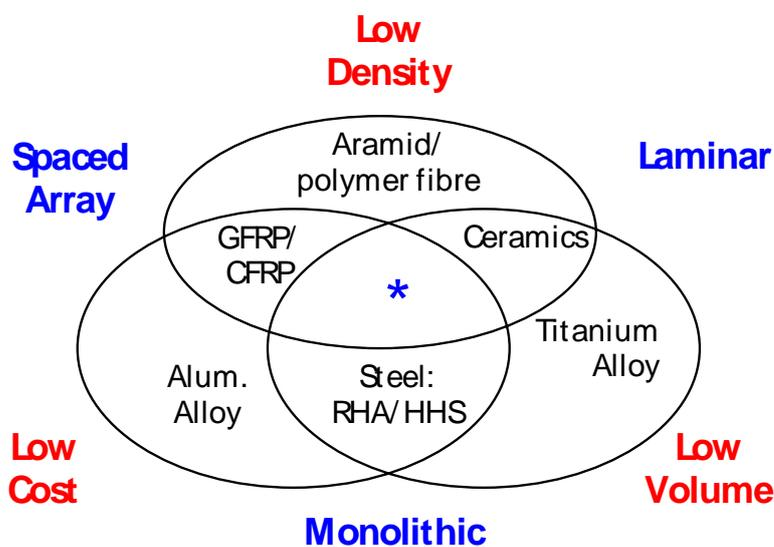
Figure 2: Venn plot showing typical armour materials arranged according to the constraints of weight, thickness and cost. Superimposed in blue are three generalised armour design types, also arranged to the same constraints.
