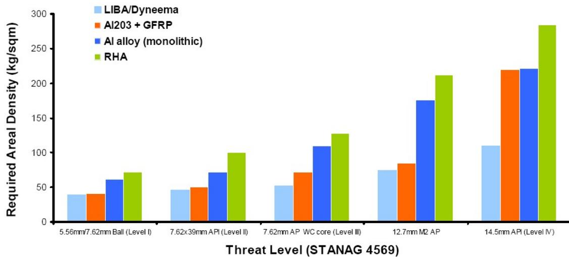
Figure 3: Weight (areal density) requirements for different armours to meet various bullet threat levels (Levels I-IV of STANAG 4569)
