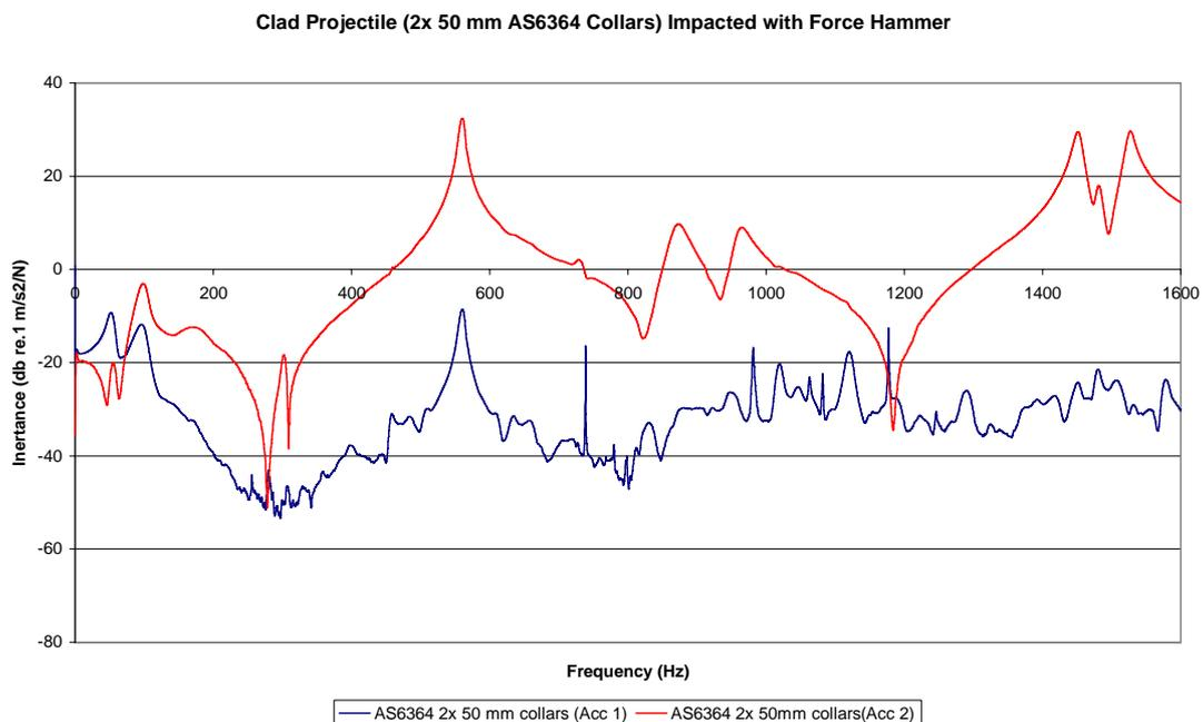
Figure 9: Fourier transforms of the input signal received by the collar and the output signal transferred to the munition
