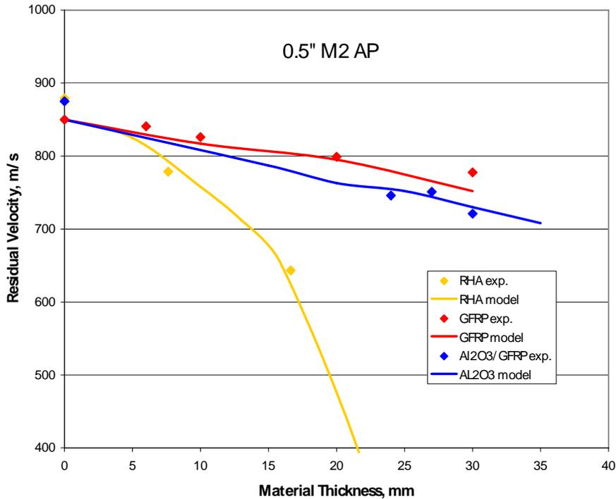
Figure 6: Modelled residual velocity curves for RHA (yellow), Glass fibre (GFRP – red) and Alumina ceramic/GFRP (blue). Experimental data points are also shown, validating the modelling results.
