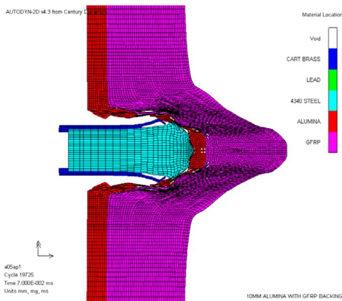
Figure 5: 0.5" M2 AP impacting a laminar ceramic/fibre composite armour system. The model depicts the erosion of the AP bullet tip.
