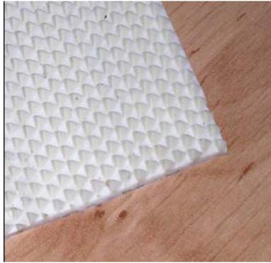
*Figure 7: A sheet of formed polymeric shock absorbing material*
