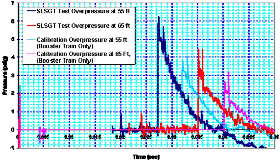
Figure 19. Overpressure record for SLSGT of Propellant F, Overlaid with Booster Calibration Shot
