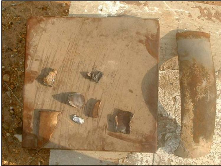
**Figure 17. Typical Post-test Photograph of the Witness Plate and Fragments for a "Passing" Reaction.**
