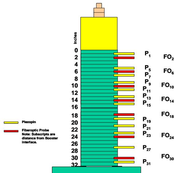
Figure 12. Test Setup for SLSGT of Propellant C.
