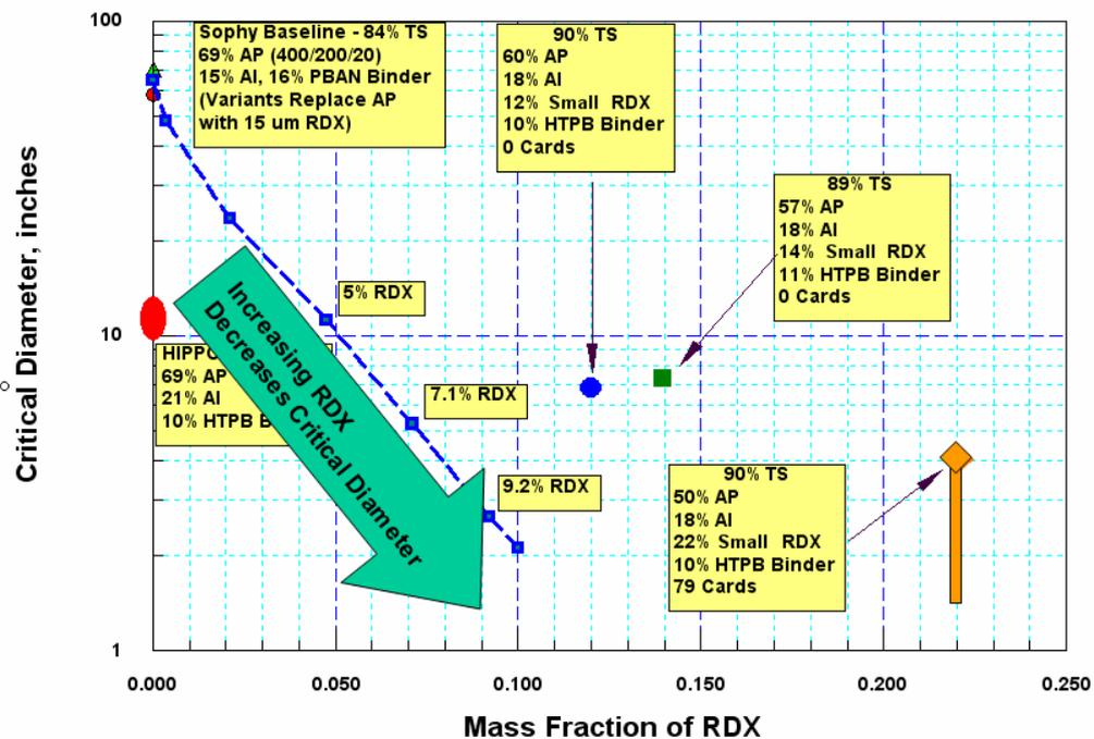
Figure 23. Effect of Increasing RDX on Critical Diameter
