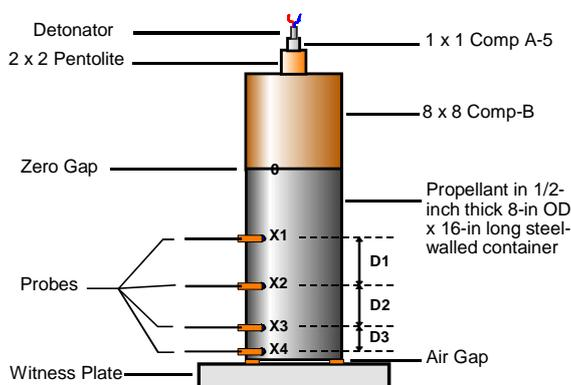
Figure 7. EXTEF 16-inch Length Acceptor, Super Large-Scale Gap Test
