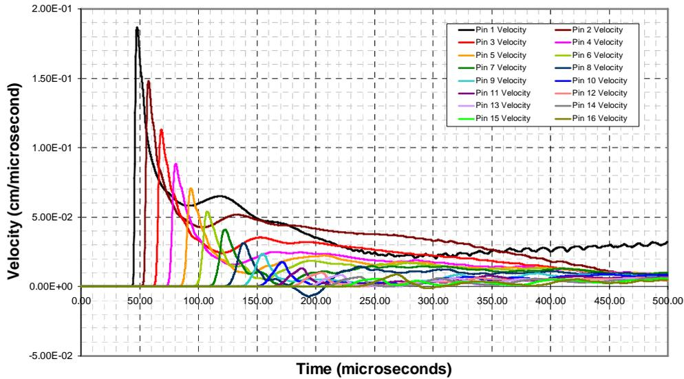
**Figure 21. Hydrocode Model of the SLSGT with Inert Polyurethane Rubber Acceptor, Acceleration at Pin Locations**
