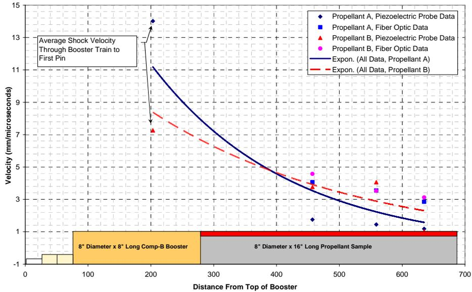
Figure 8. Shock Velocity Data for the 16-Inch Super Large-Scale Gap Test with Four Probe Locations
