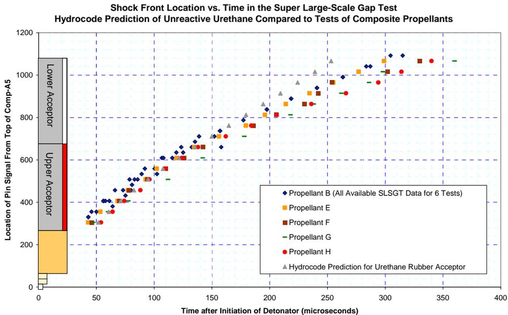
**Figure 22. Hydrocode Prediction of Pin Response for Polyurethane Acceptor Compared to Know Composite Propellant Response**
