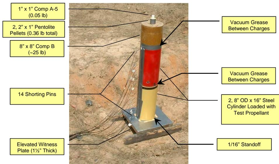
**Figure 16. Typical Aerojet Set-up of the 32-inch Acceptor, Super Large-Scale Gap Test.**
