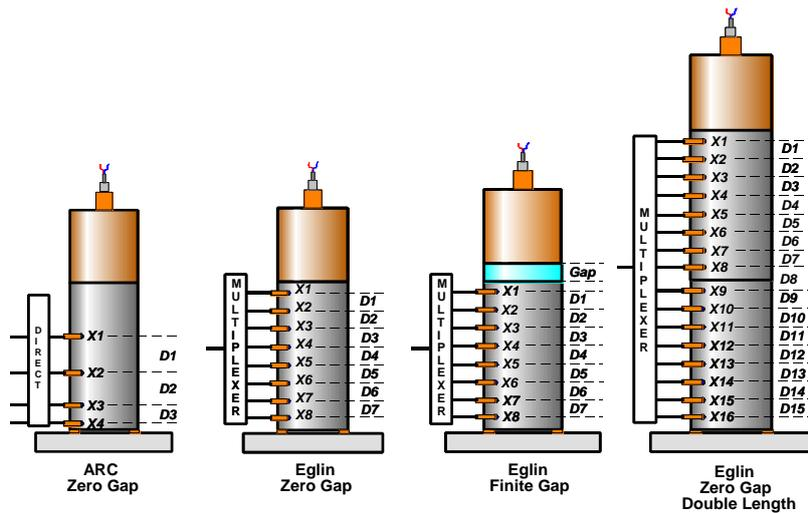
Figure 9. Four Different Types of Super-Large Scale Gap Tests Performed on Propellants A and B.
