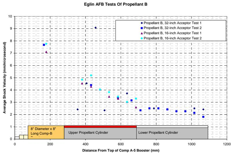
**Figure 11. Super Large-Scale Testing of Propellant B at Eglin AFB (Velocity vs. Distance)**
