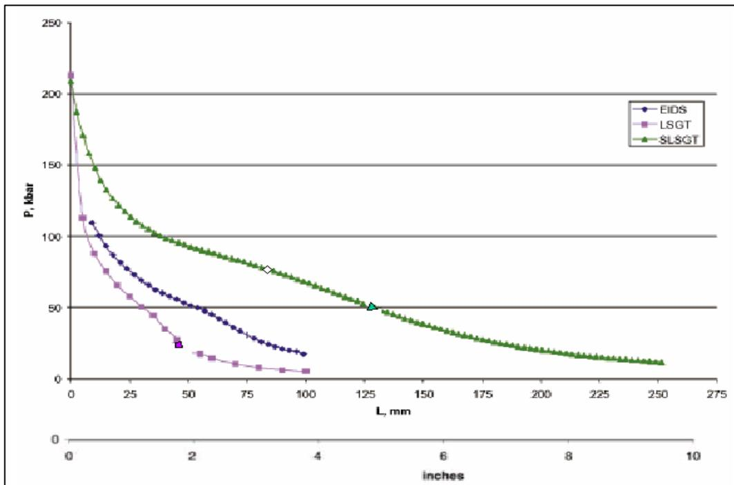
**Figure 6. Input Shock into the Acceptor vs. Attenuator Thickness for Three Gap Tests**
