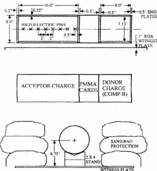
Figure 4. Test Set-up for the 8-inch "super gap test"
