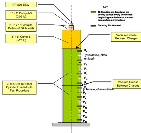
**Figure 14. Current Aerojet Set-up for the Super Large-Scale Gap Test.**
