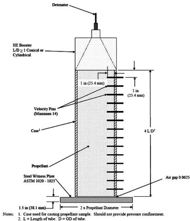
Figure 2. Unconfined Critical Diameter Test Fixture
