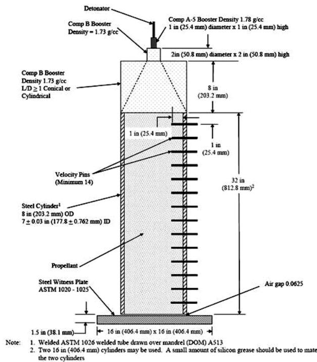
Figure 1. Super Large-Scale Gap Test Fixture
