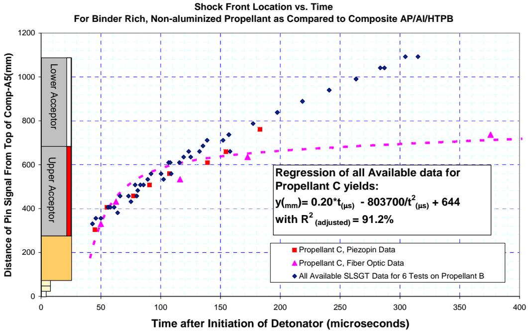
**Figure 13. Piezoelectric Pin Data and Fiberoptic Probe Data for Propellant C SLSGT**
