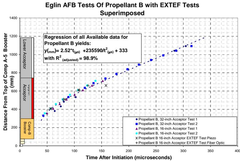
**Figure 10. Super Large-Scale Testing of Propellant B at Eglin AFB. (Position vs. Time Data)**
