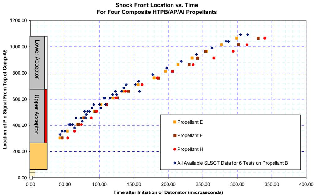
**Figure 18. Compiled Super Large-Scale Gap Test Data for 4 Composite AP/AI/ HTPB Propellants**
