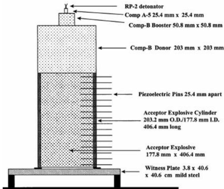
Figure 5. Test Set-up, Super Large-Scale Gap Test (circa 1999)
