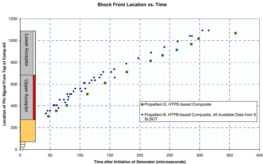
Figure 20. Comparison of Super Large-Scale Gap Test Data for HTPB-based and HTPE-based propellants
