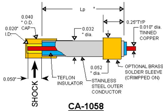
**Figure 15. Schematic of Dynasen Shorting Pin Model CA-1058**
