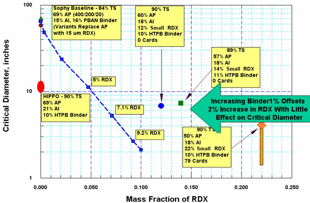
Figure 24. Effect of Increasing Binder on Critical Diameter
