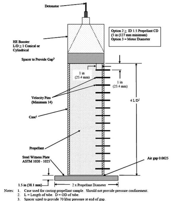
Figure 3. 70 Kilobar Motor Confinement Gap Test Fixture
