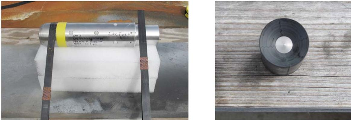
Figure 7. Orientation of warhead on left. Fragment assembly on right.
