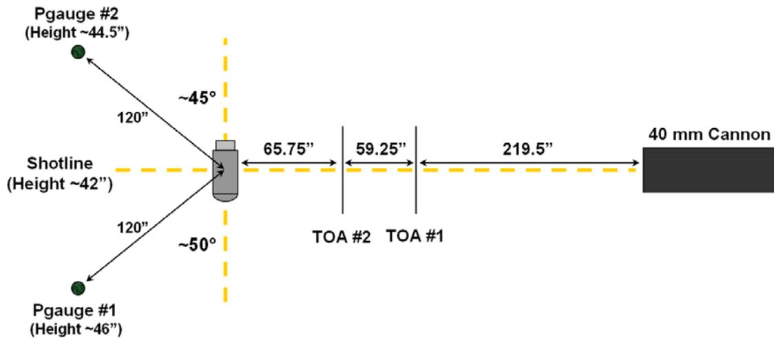
Figure 8. Test setup diagram.
