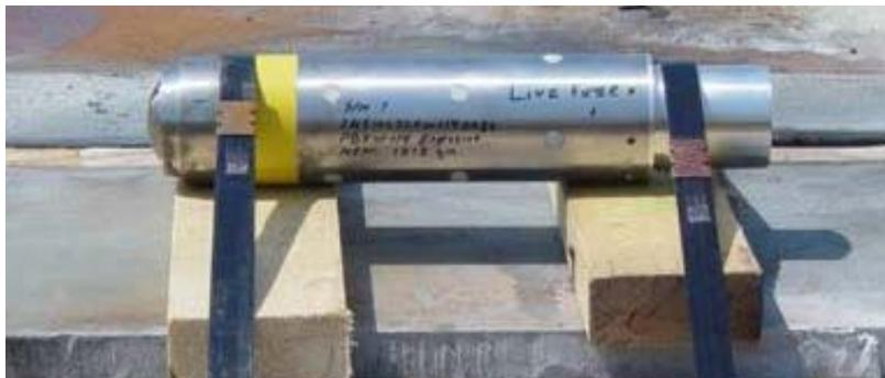
Figure 4. 2.75" Warhead ready for bullet impact testing.
