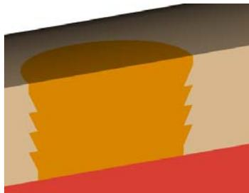
Figure 2. Close up of vent plug geometry.
