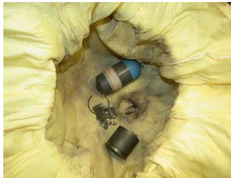
**Figure 3 - Ignited Cartridge in Kevlar® Liner in PA120 Box**
