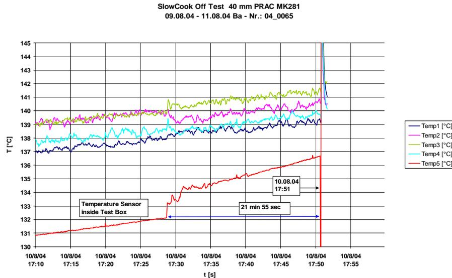
**Figure 6 - Temperature /Time Profiles in Slow Cook-Off Testing of MK281 Cartridges using M2 Propellant**
