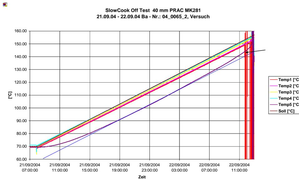
**Figure 7 – Temperature/Time Profiles in Slow Cook-Off Testing of MK281 Cartridges using F15080 Propellant**
