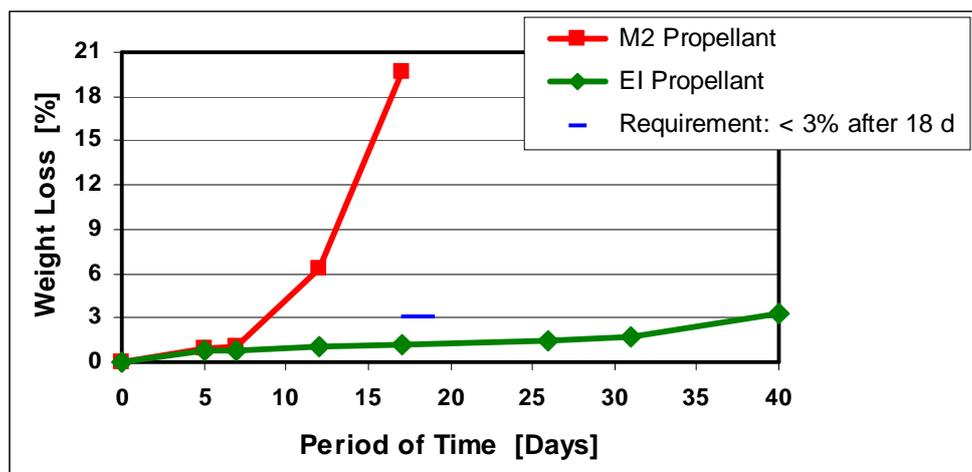
Figure 4 - German STANAG 4170 Qualification Testing of M2 and EI Powder
