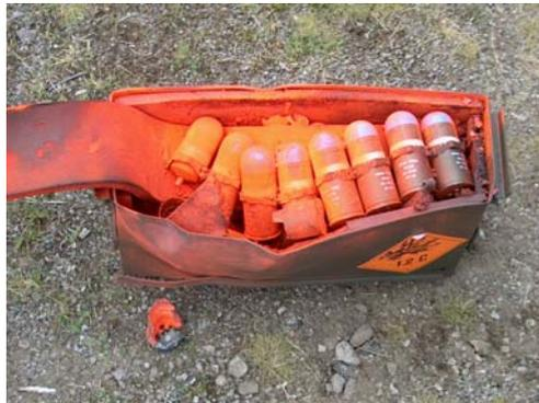
**Figure 5 - Lengthwise Bullet Impact on PA120 Box**
