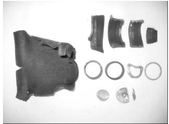
Photo 5. Test Vessel of H-2 after the Test
