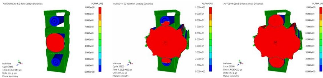
Figure 4 – Sympathetic reaction of missiles within a stack
