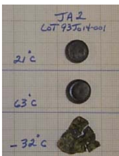
Figure 7: Remains of JA2 Specimens Tested at 21 °C, 63 °C, and -32 °C Mechanical Testing Results:
