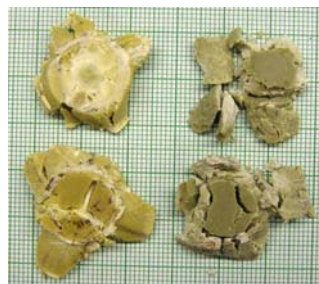
Figure 21. ETPE Lots 8288RR1 and 8194R1 Specimens Tested at -32° C
