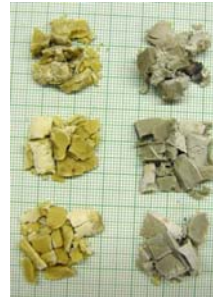
Figure 28. ETPE Lots 8194R5 and 8288R5 Specimens Tested at -32° C
