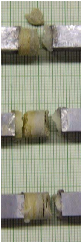
Figure 31. Tested Specimens of Co-Layered Material at 21° C. Failure did not occur at layered seam.
