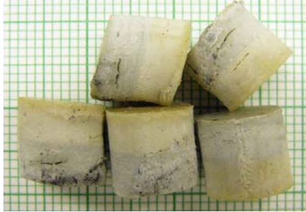
Figure 29: Co-layered Propellant Test Specimen
