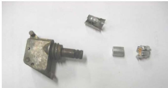
Figure 7: Functioned Fuze with Triazide, PBXN-5 Lead and PBXN-5 booster
