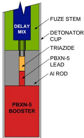
Figure 6: C70 cup loaded with primary and PBXN-5
