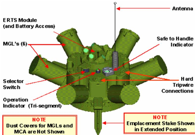
**Figure 1: Spider Munition Control Unit (MCU)**
