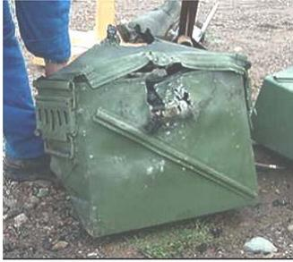
**Figure 8: Post SD examination showing fragment perforations**
