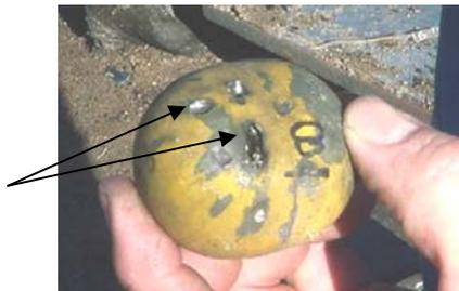
**Figure 9: Post SD examination showing fragment perforations in acceptor grenade**
