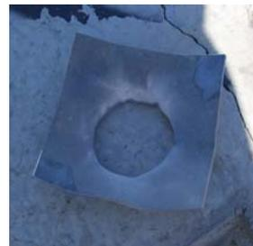
*Figure 9 (a) UN Series 2 Gap Test Set-up prior to firing, (b) witness plate no reaction and (c) holed witness plate after booster removed from pure DNAN charge.*
