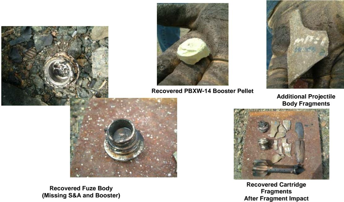
Figure 4: Fragment Impact Results for 81mm Mortar, Test #2 – Type IV Reaction
