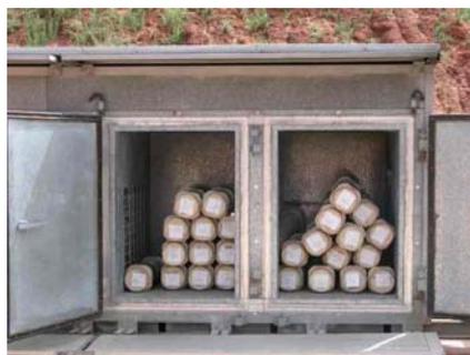
Fig. 1 - Accelerated ageing oven storage
