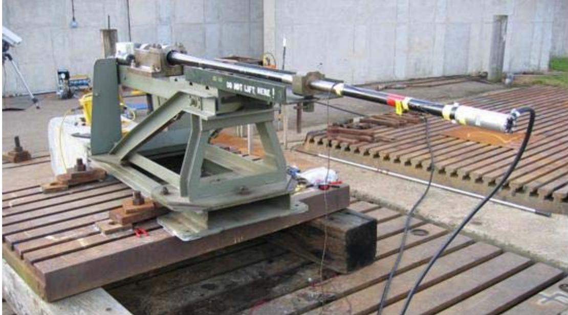
*Figure 3: 30mm calibre, alternative lower velocity gun system*
