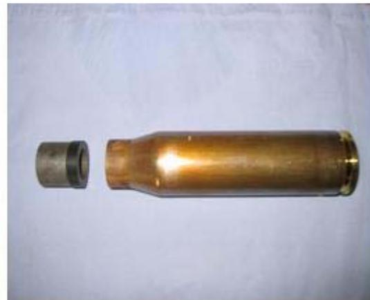
*Figure 5: 30mm FSP and case ammunition*
