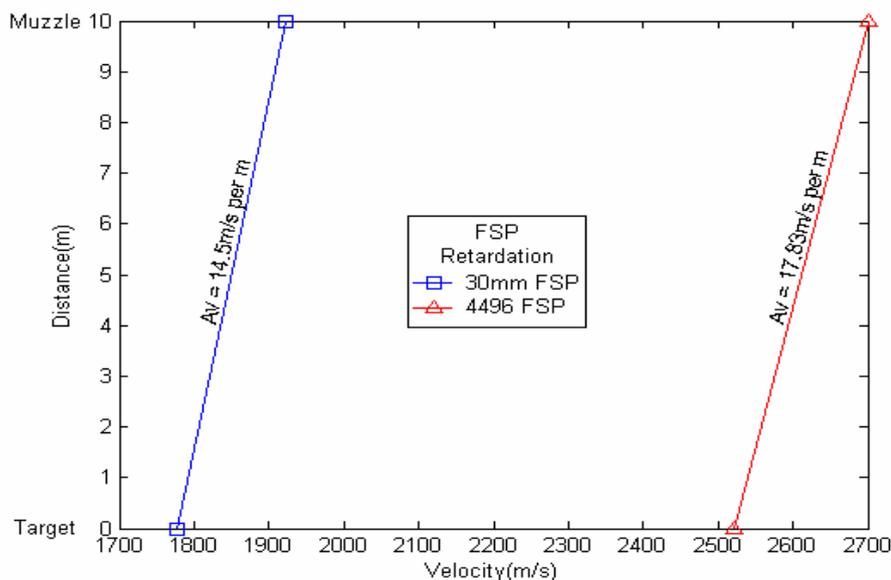
Graph 1: Retardation over a given muzzle to target distance of 10m
