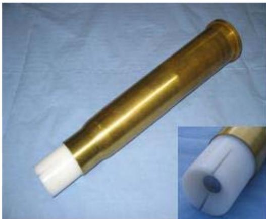
*Figure 4: Assembled STANAG 4496 ammunition*
