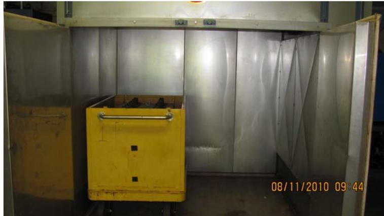
Figure 2 – Metal Part Pre-Heat Oven
