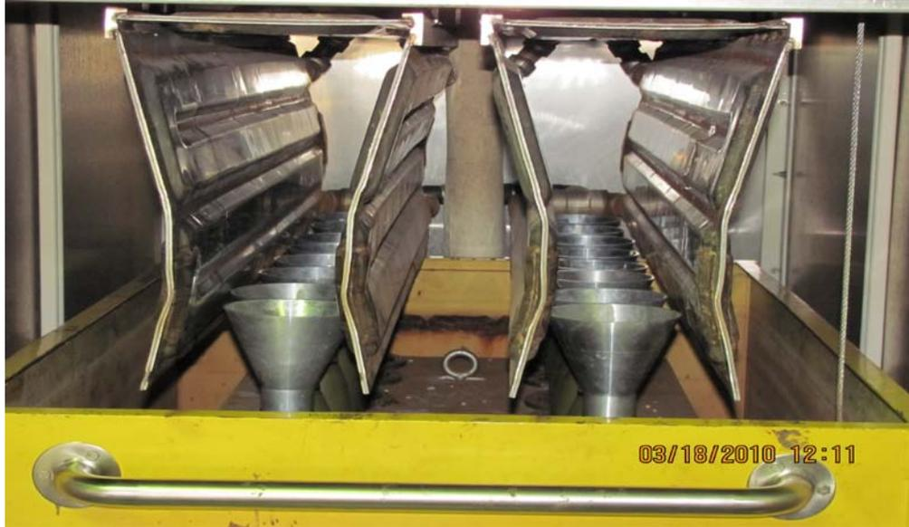
Figure 5- Control Cooling Oven and Load Cart
