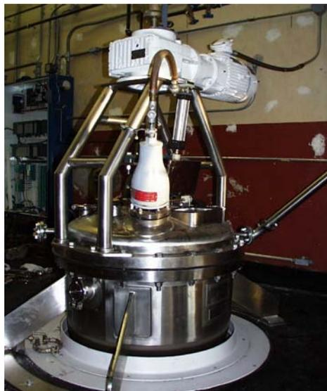
Figure 3 – 50 Gallon Melt Kettle
