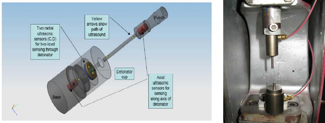
**Figure 10 Primer press which was instrumented using ultrasound technology.**
