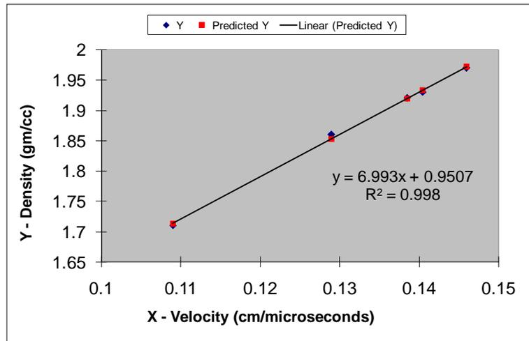
**Figure 8 Relationship between Ultrasonic Velocity and Density.**
