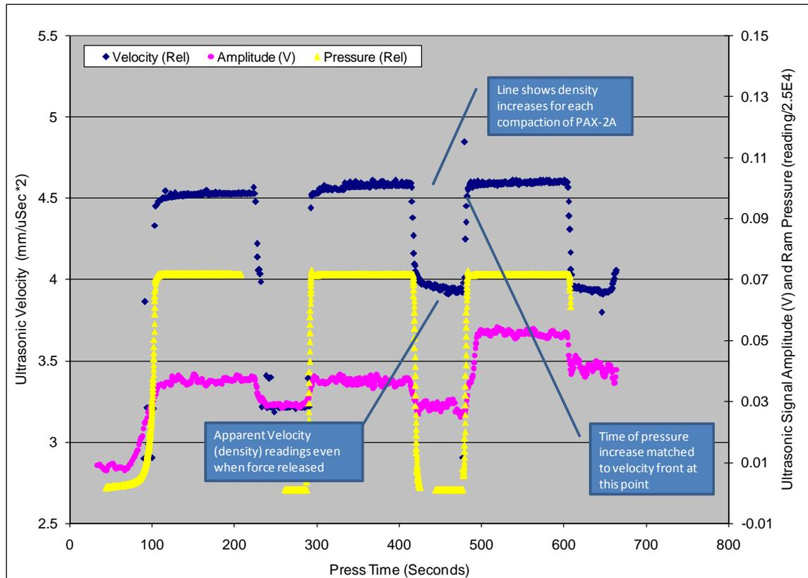
**Figure 9 Results of PAX 2A Pressing Using 81mm Ultrasound Die Set.**
