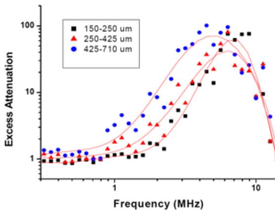
**Figure 4** Measured ultrasonic attenuation for three slurries with different particle size ranges
