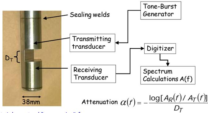
Stainless steel "gap probe" for immersion into the slurry vessel
