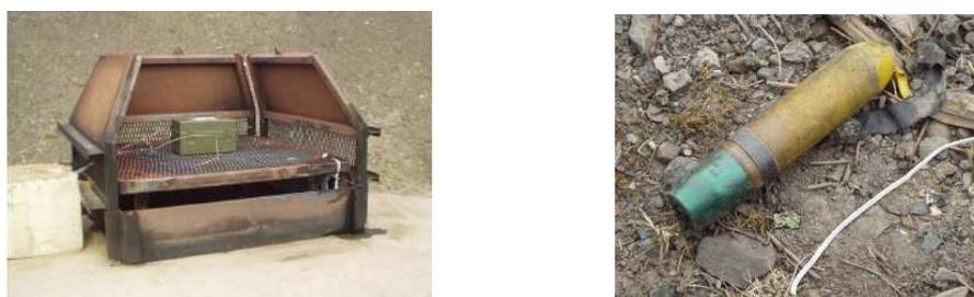
Figure 11: 40 mm cartridge before and after FCO test
