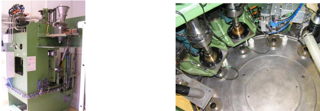
Figure 4: Press for 40CTA ammunition
