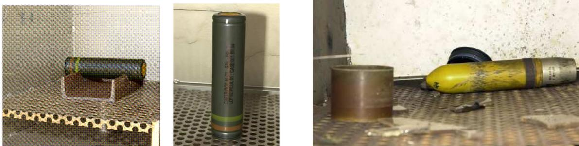
Figure 10: 40 mm cartridge before and after SCO test
