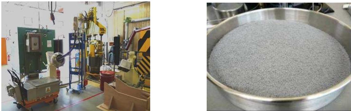
**Figure 3: Coating apparatus in Nexter Munitions facility and view of XP3264<sup>®</sup> agglomerates**
