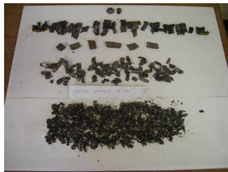
**Figure 13: Fragmentation of 40 mm cartridge (static firing test)**
