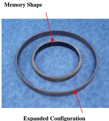
Figure 7. Comparison between expanded and memory shapes of SMP composite ring
