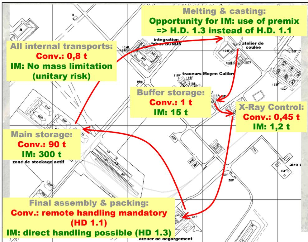
FIGURE 3: Example of industrial fluxes in Nexter's plant, the maximum acceptable weight of explosive is indicated for each workshop with comparison between conventional and IM shells.
