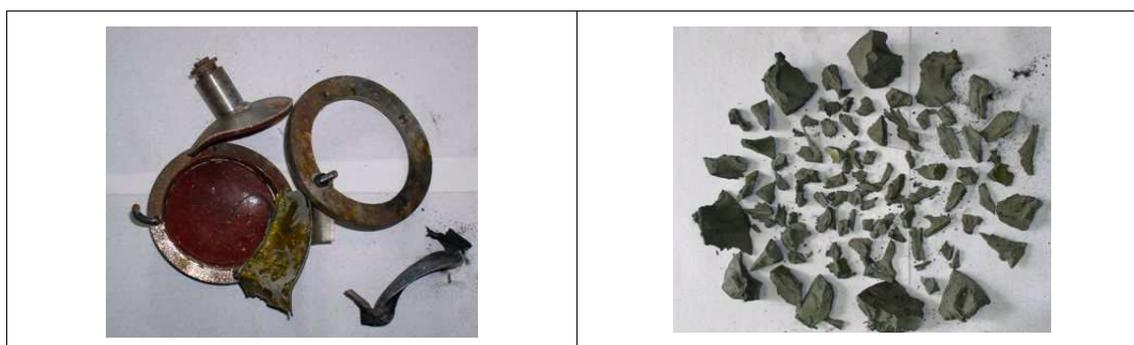
Almost 40 % (in mass) of the tested EM was recovered unburned (which is a necessary under estimated value, given as a slight indication). Neither metallic fragments nor blast overpressure was generated (no peak on pressure signal), which is another proof of moderate reactivity level of the Azalane<sup>®</sup> propellant.
