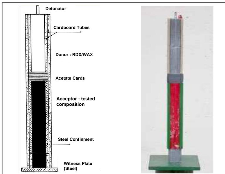
The Gap Test results on Azalane<sup>®</sup> propellant were the followings:
