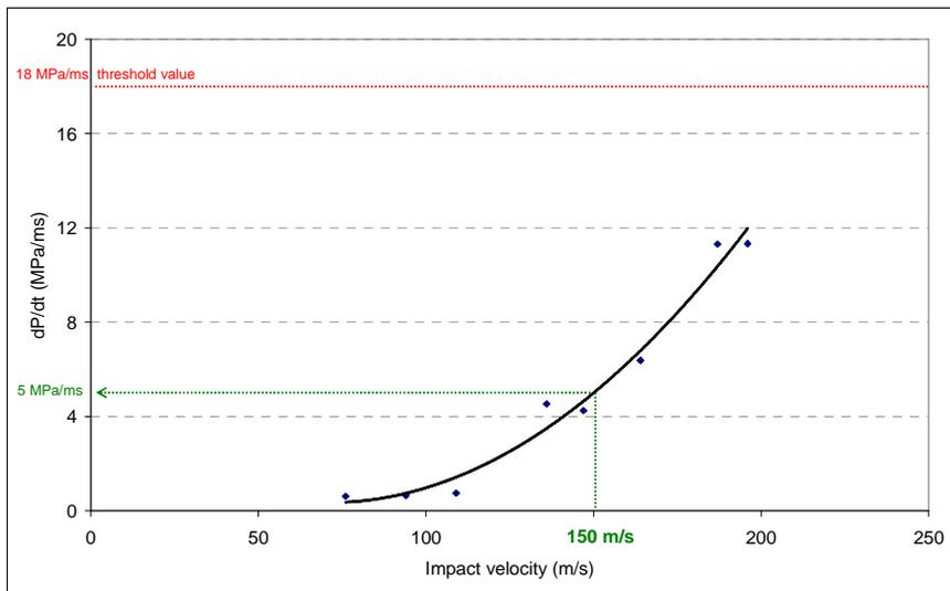
Due to its good mechanical properties, the threshold value of  $(dP/dt)_{\max} = 18 \text{ MPa/ms}$ , is reached beyond impact velocities that have been tested. Moreover, this impact velocity is considered as a key value, and thus exhibits great margins, when compared to the common reference value defined at 150 m/s. Classical HTPB composite propellant exhibit very similar impact velocity when  $(dP/dt)_{\max}$  reaches 18 MPa/ms.
