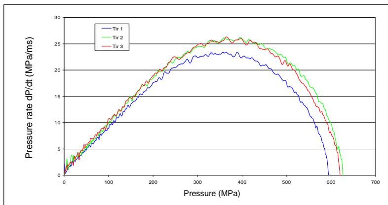
Analyzing these results (friability and high pressure combustion test), one can assess that this composition have a great potential for no violent reaction when submitted to bullet impact threat. Indeed, bullet impact trials have been performed to confirm this point.
