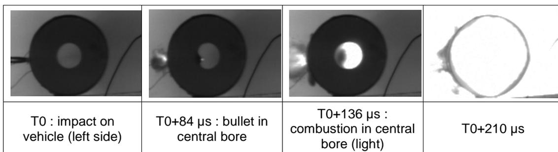
Like for the previous test, neither metallic fragments are generated nor blast overpressure is measured.
