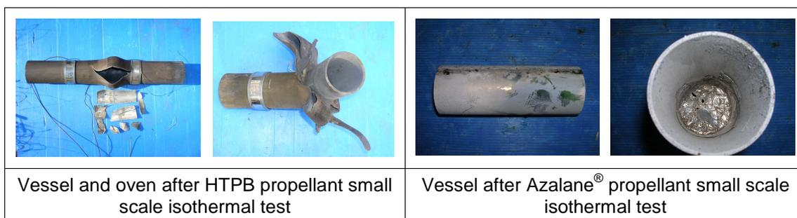
Further tests including slow heating standard tests will have to be performed in order to achieving IMness for rocket motors made of aluminized GAP based propellant.
