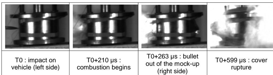
Just after impact on the mock-up, combustion (lights on high speed camera pictures) is observed, before the bullet gets out of the vehicle. Then, the up lid opens; with pressure increase in the bore area up to a few tens of bars is measured just before opening. Then, the next step is the mock-up pneumatic explosion.
