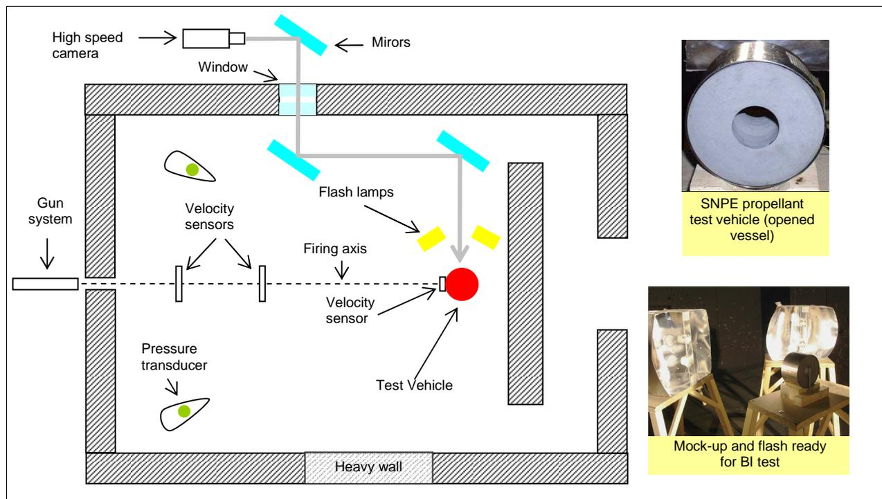
The standard SNPE test vehicle, specially designed for rocket propellant testing is there used. A picture is shown on previous figure. The structure is constituted of a cylinder (Inner diameter: 158mm – Length: 100mm), with two 5 mm thick lid, closed with tie rods, made of standard stainless steel. The mock-up is filled with the propellant to be tested which has a cylinder central bore of 52 mm diameter,
