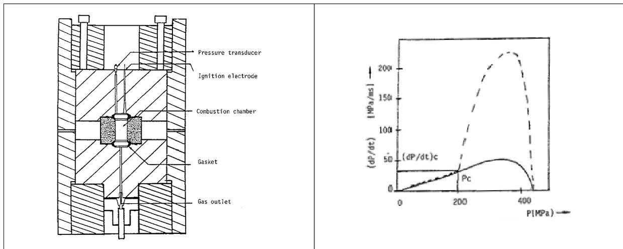
This test is one of the most pertinent way to quantify the damage through the specific surface, induced by a mechanical loading. It gives a relation between mechanical loading and reactivity, in other words violence of reaction. Indeed, it allows quantifying the specific surface in the sense of the violence of reaction.
