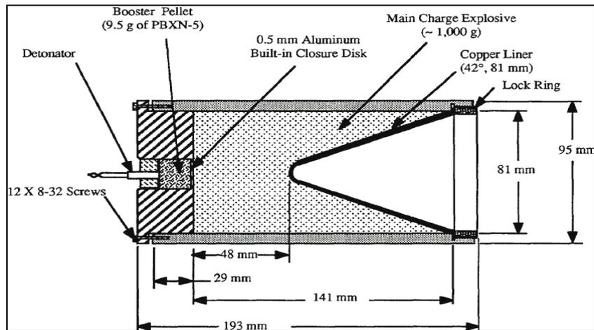
Figure 4: Example of GTU Drawing - 3.2" Generic Shaped Charge Testing Unit (BIRD v1.2)
