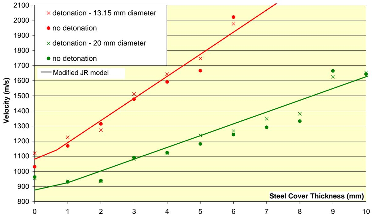
Figure 13: Flat-Ended Fragment Impact Tests on Steel Covered Rowanex-1001 Blocks Modified Jacobs-Roslund Modelling Calculated from these Tests
