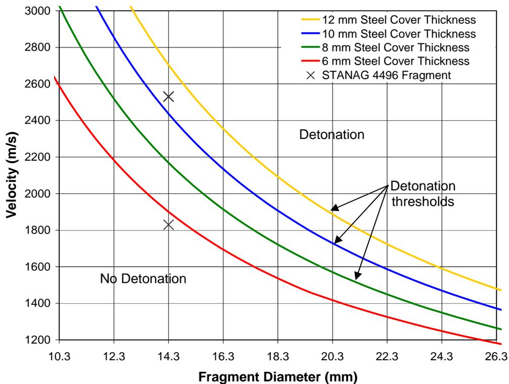
Figure 14: TEMPER Simulation of STANAG 4496 Fragment Impact on PBXN-110 Blocks Covered with Steel
