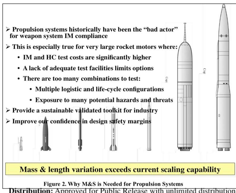
Propulsion M&S is essential for reasons such as those summarized in **Figure 2**. For very large missiles, full-scale testing is costly and may be impracticable due to the lack of sufficiently large instrumented facilities. M&S is an enabler. It can help establish scalability for reliable sub-scale testing of very large motors. For all motor sizes, it strongly complements testing, which alone cannot feasibly cover all the combinations of system
